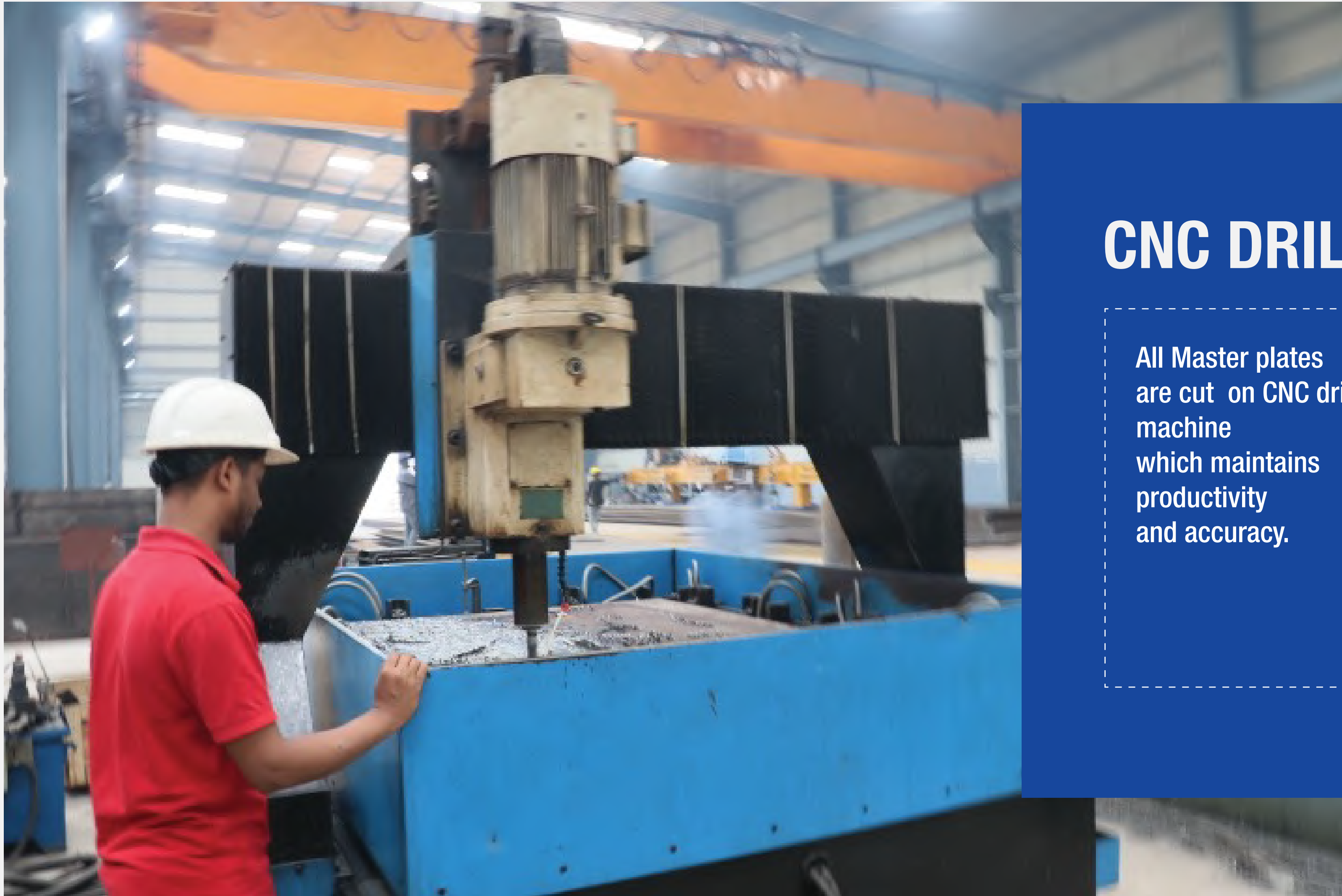
CNC DRILLING MACHINE WITH BED SIZE 1600MM X 2000MM UPTO 40MM HOLE DIAMETER
